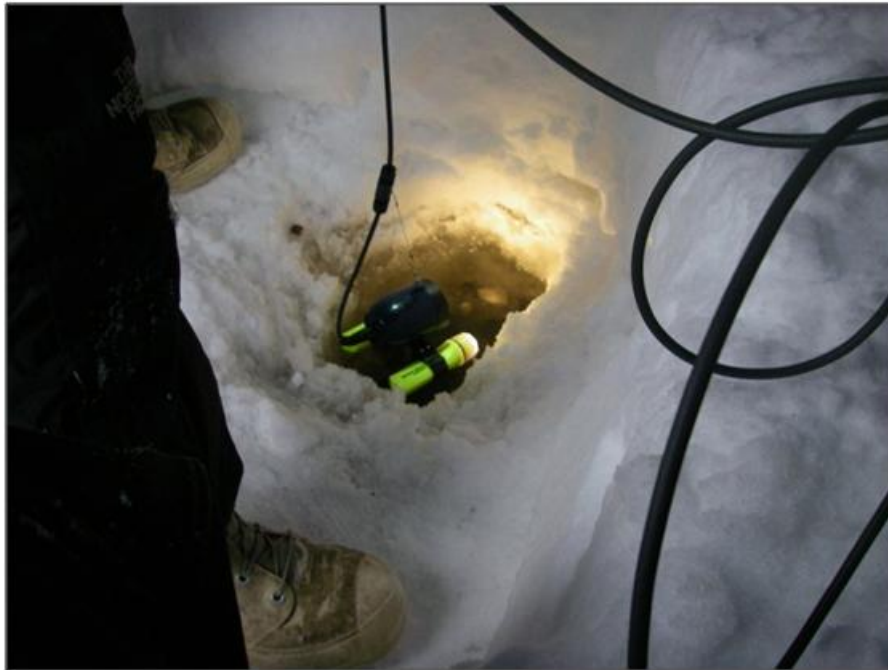
FIGURE 2-6: CAMERA BODY AND ATTACHED LIGHT SOURCE BEING LOWERED THROUGH THE ICE OF STREAM 2003.
